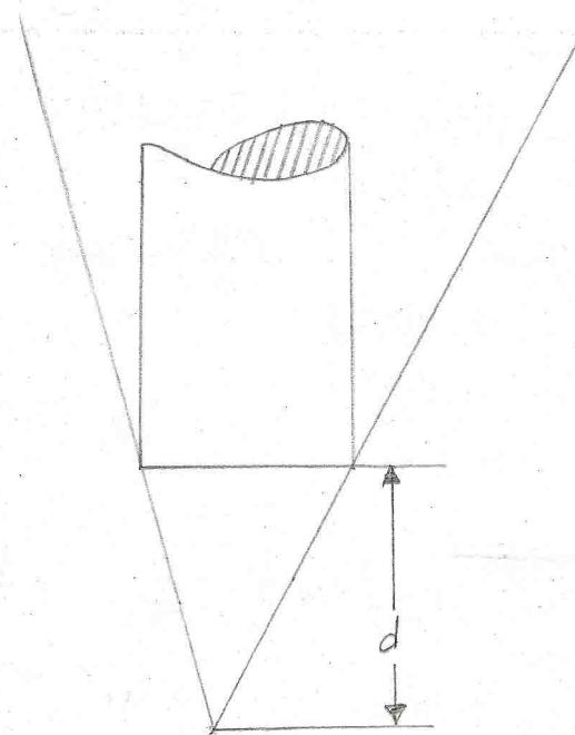
(iii) Depth of indentations, caused by indenter in Rockwell Hardness
