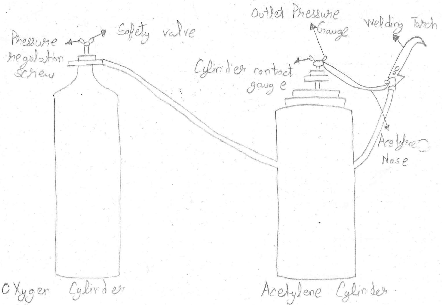
Oxy - Acetylene Welding
